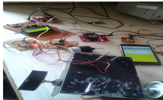
Fig.12 when there is an obstacle near to it, then IR Sensor activities automatically the bus will be stops
