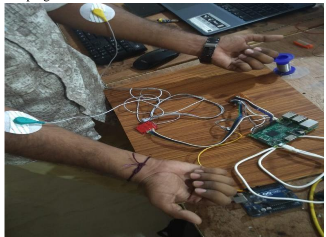
Fig 6. Hardware overview of patient health monitoring system
