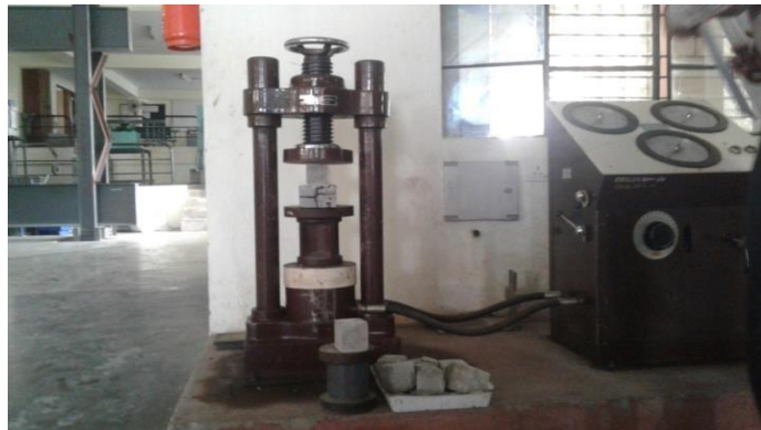
Figure – 5.1 Compressive tests on concrete cube.
