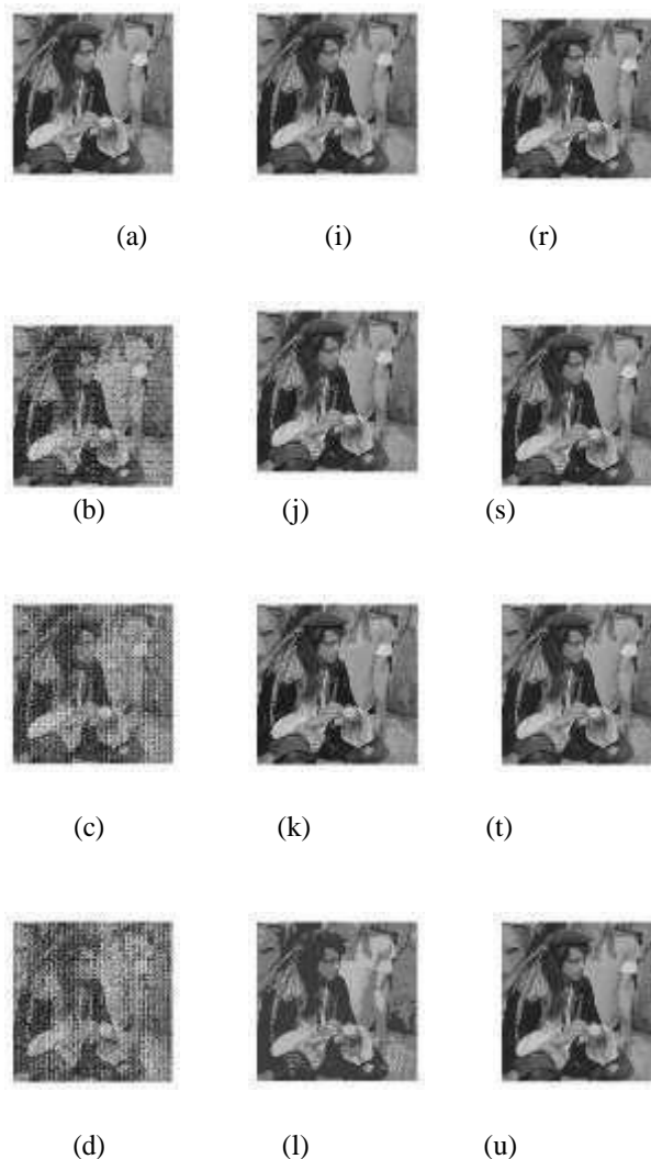
Fig. 11: Reconstructed benchmark image [13, 14] for varying ET using BWA-DCT (a-d), TEA-DCT (i-l), and proposed DCT (r-u) architectures.
